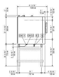
Cold Water inlet 1 (cleaning) CWII Cold Water Inlet 2 (steam CWI2
